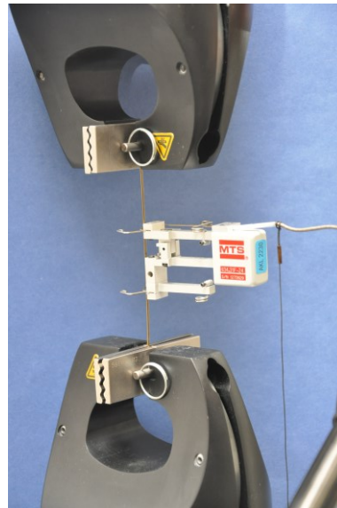
Fig. 2 Detail of NiTi wire sample attached in pneumatic jaws and MTS extensometer
