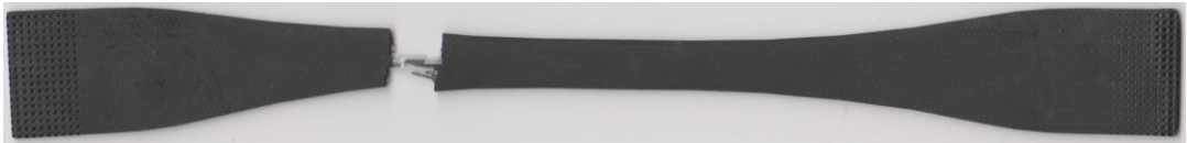
Fig. 3 Ruptured specimen. Fracture in the shoulder region
