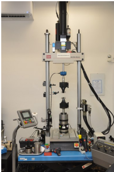
Fig. 1 Testing system Mini Bionix 858.02, load cell and pneumatic jaws
