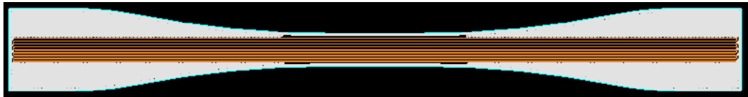
Fig. 4 Specimen with long fibres arranged in part bounded by gage region
