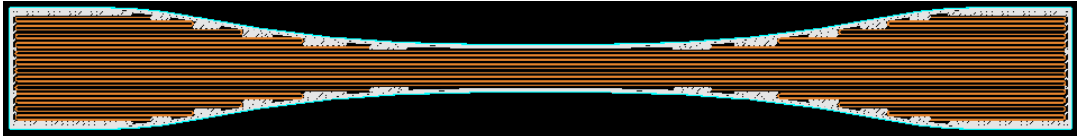
Fig. 2 Specimen with long fibers arranged across the entire lamina plane
