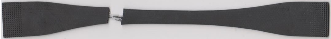
Fig. 3 Ruptured specimen. Fracture in the shoulder region
